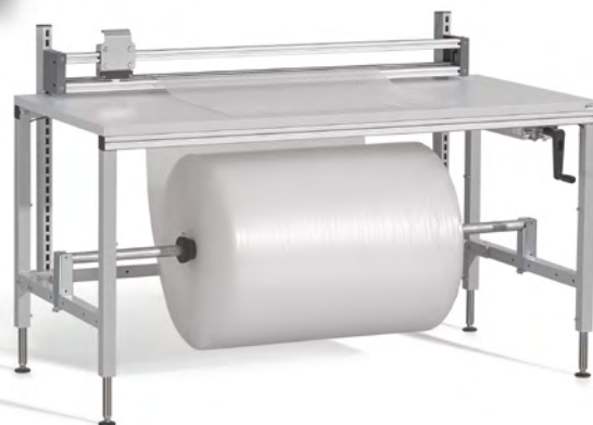
Height-adjustable table with a film unwinding and cutting device, operated by a hand crank – ideal for packaging exhibits.
